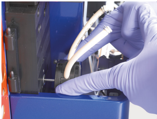
Figure 7.25: Detachment of the pump head.
