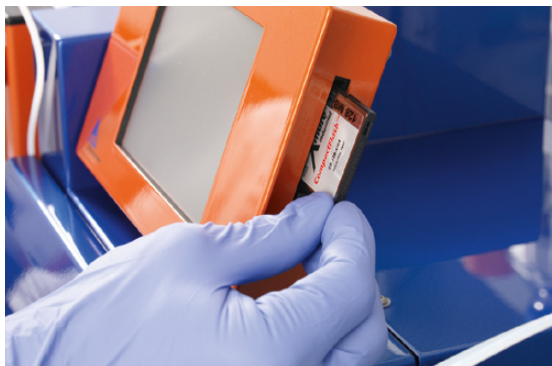
Figure 2.7: Insert the software memory card.
