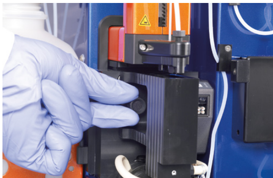
Figure 7.20: Dismantle the washing station.
