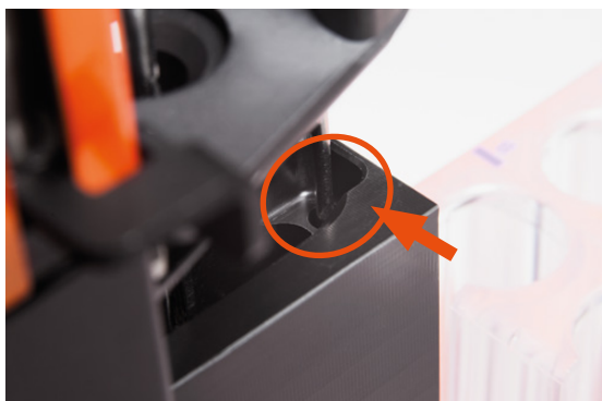
Figure 5.5: NEG needle in the washing station.
