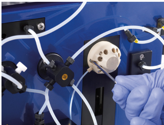
Figure 7.17: Unscrewing the dilutor valve's socket screws.
