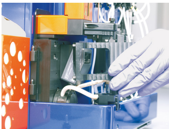
Figure 7.21: Dismantle the washing station.
