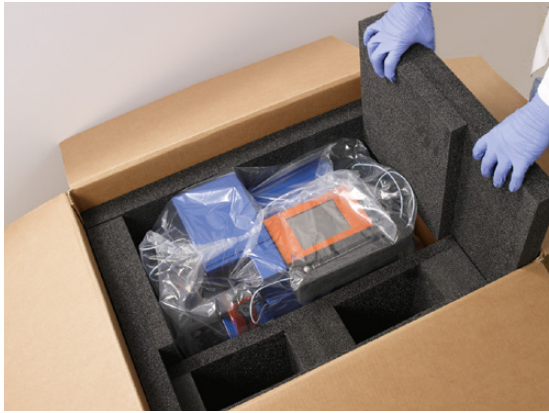
Figure 2.3: Remove the foam packaging from both sides of the autoMACS Pro.
