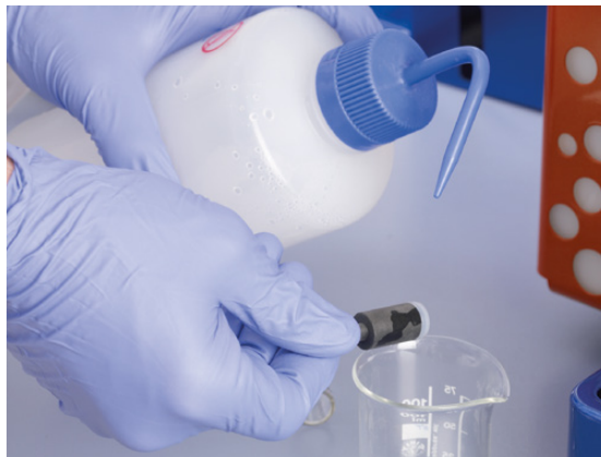
Figure 3.2: Humidify the plunger.
