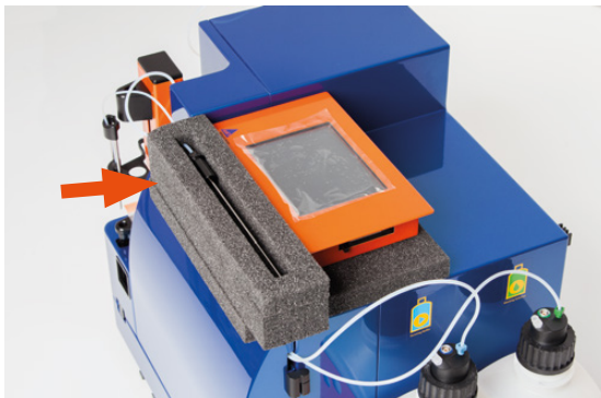
Figure 2.5: Remove the uptake needle from the foam packaging (arrow).
