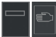
Figure 4.7: MACS MiniSampler status graphic. Left: The MiniSampler was successfully installed. Right: No MiniSampler was detected.
