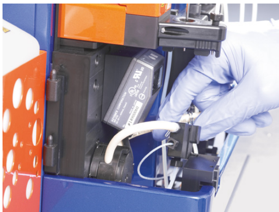
Figure 7.23: The draining tube is attached.
