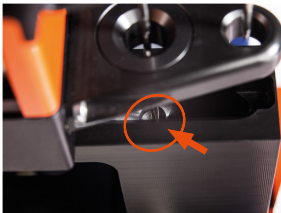
Figure 5.3: Uptake needle position in the washing station (arrow).
