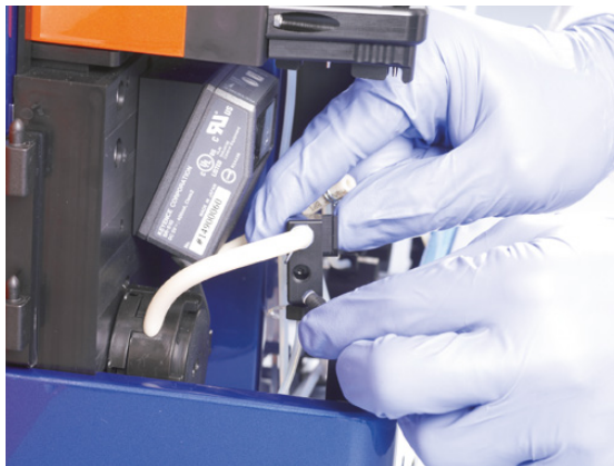
Figure 7.22: Removal of the waste distributor.
