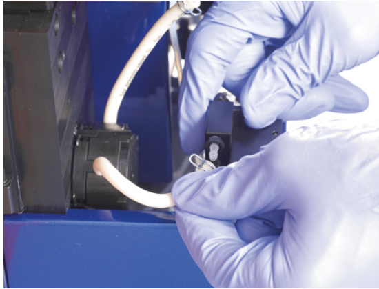
Figure 7.24: Disconnecting the tubing from the waste distributor.
