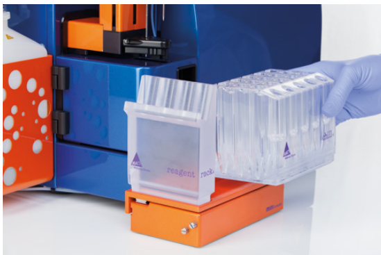
Figure 2.11 Install the Chill Rack onto the MiniSampler.
