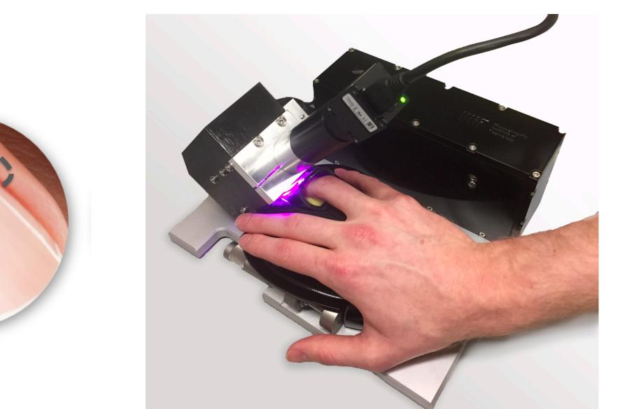
Our idea: Estimating neutropenia noninvasively with a portable optical device
